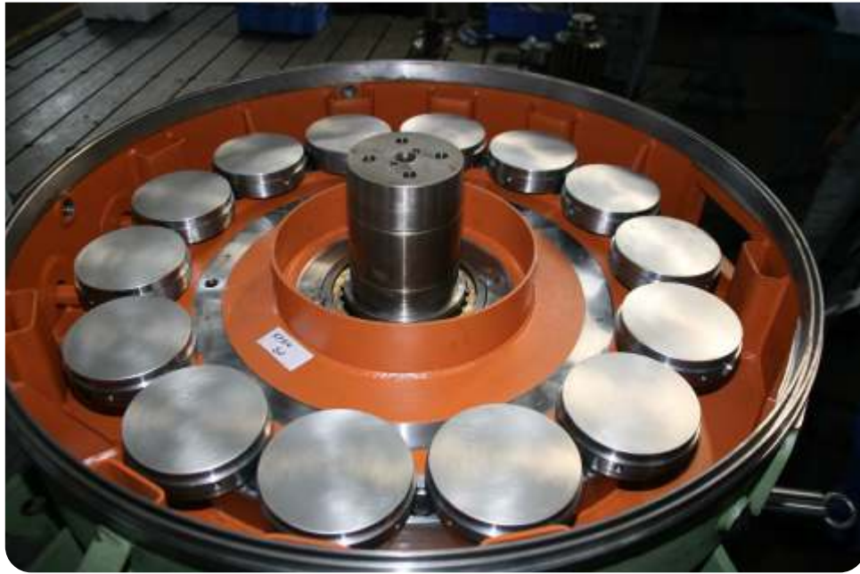
Axial thrust bearing of gearbox unit B1PV 180
